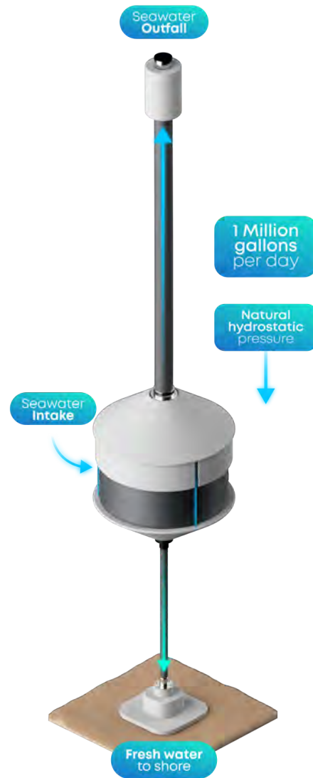
Figure 2 | OceanWell 1MGD pod design
